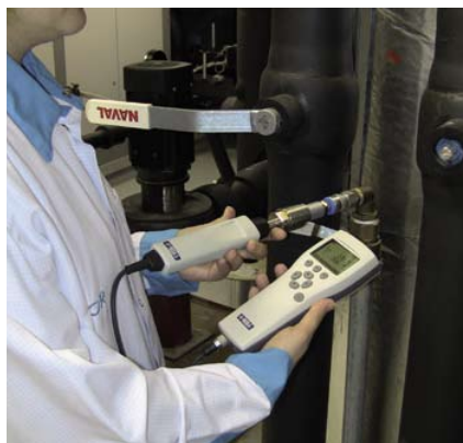
Lightweight hand-held meter DM70
