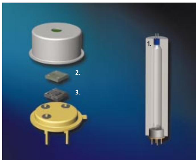
A cutaway of Vaisala's CARBOCAP® CO 2 sensor: (1) an InfraRed source, (2) an F-P filter and (3) an IR detector.
