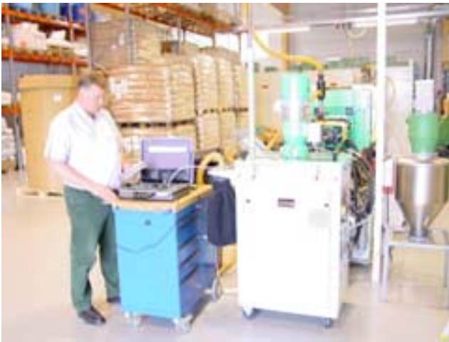
The Vaisala DRYCAP® Portable Dewpoint Sampling System DSS70A is an easy-to-use solution for spot-checking dryer performance.
