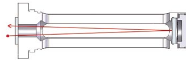
Figure 2: The passage of light in the SPECTRACAP® sensor probe used in the OMT355.
