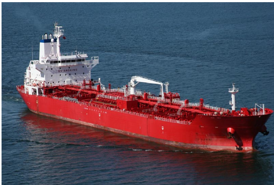
Fuel tankers are required an oxygen measurement in their on-board inerting system before they are allowed to empty their tanks at the port.
